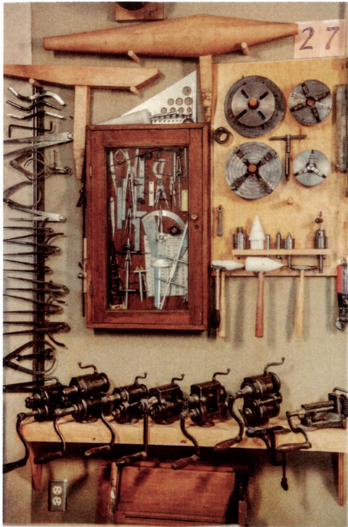
Assorted tools for measurement, edge turning, and lathe work.
